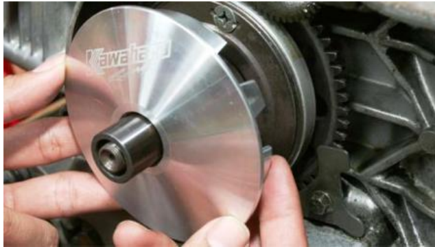
Gambar 3.7 Melepas primary sliding sheave
