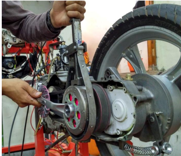
Gambar 3.10 Proses melepas clutch housing
