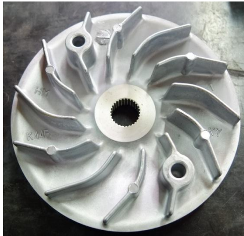
Gambar 2.2 Primary fixed shave
