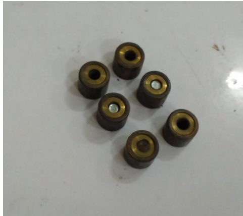
Gambar 2.4. ( primary sheave weight )
