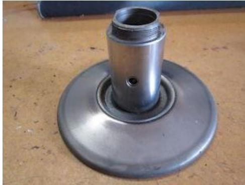
Gambar 2.7. *secondary fixed sheave*
