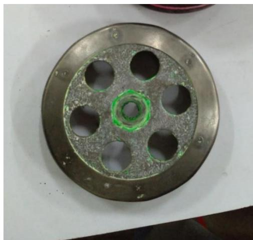
Gambar 4.11 *Clutch housing*
