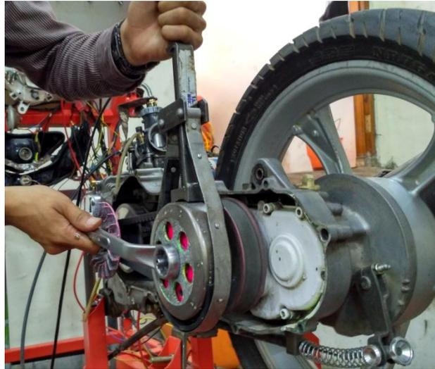
Gambar 3.10 Proses melepas *clutch housing*
