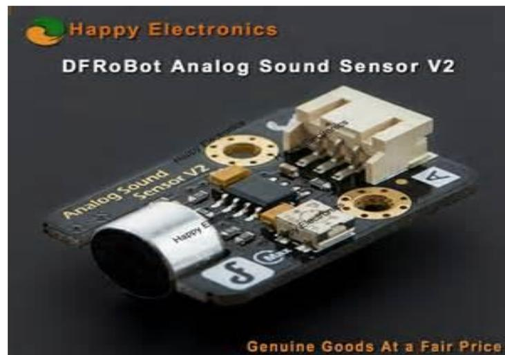
**Gambar 2.9** *Sound sensor V2*
