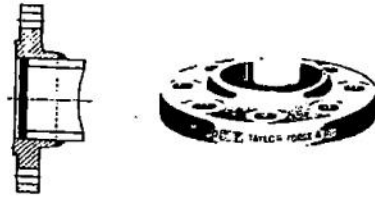
Gambar 3.8. Flange jenis SO (Slip-On)
