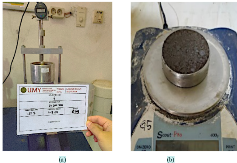
FIGURE 1. (a) Consolidation testing (b) the specimen
