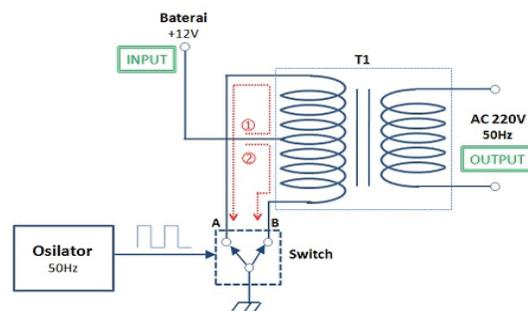
FIGURE 1. Basic structure of an inverter
