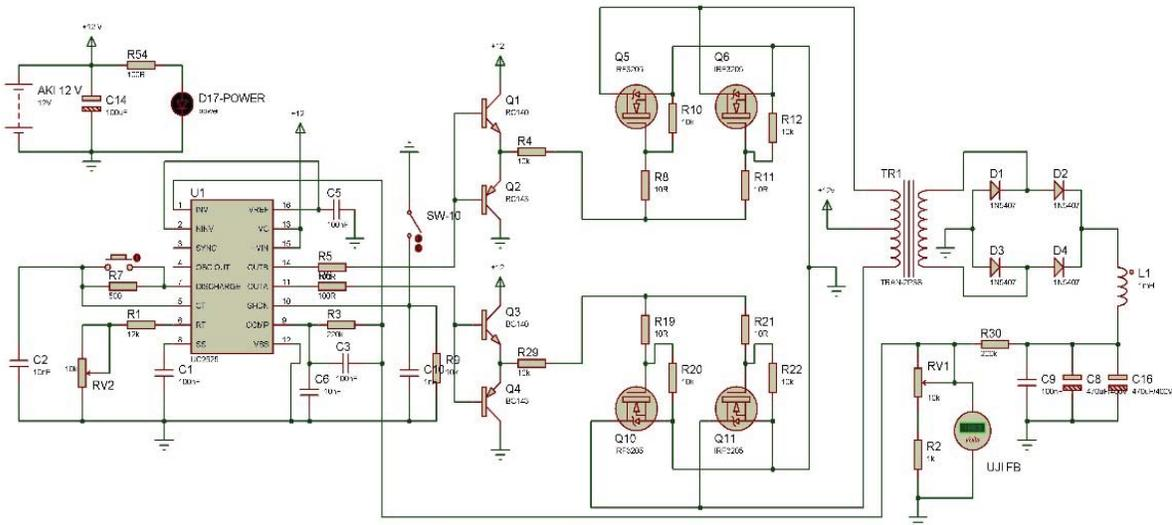
**FIGURE 6.** Test scheme of feedback voltage testing of the IC SG3525 module
