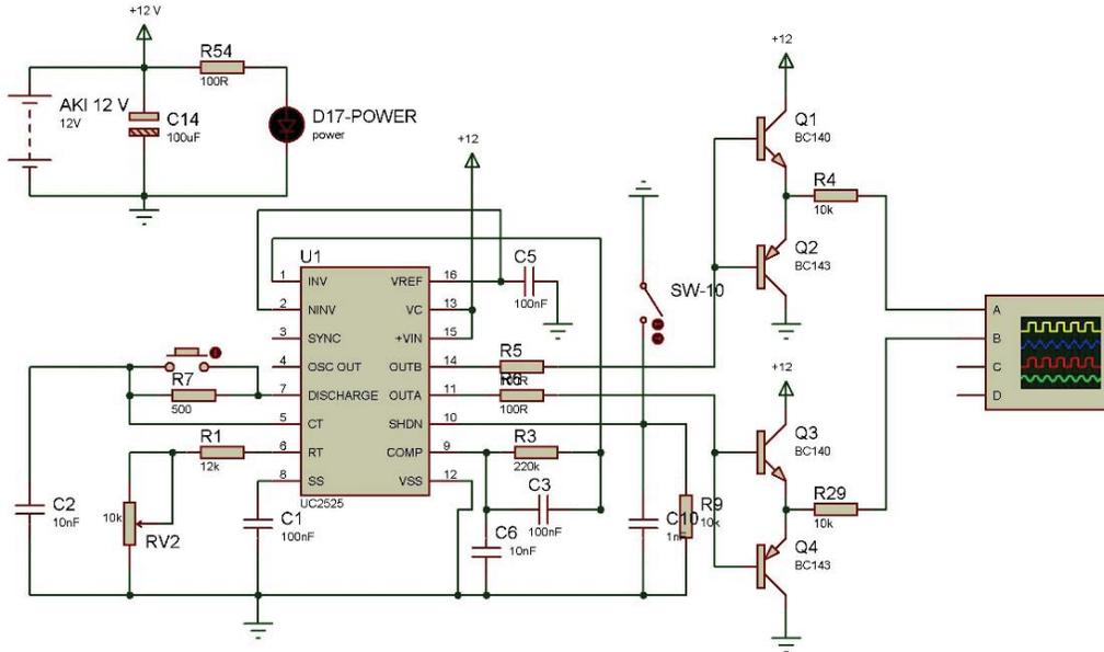
FIGURE 4. Test scheme of the IC SG3525 module
