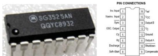
FIGURE 2. SG3525 module and its pin connection
