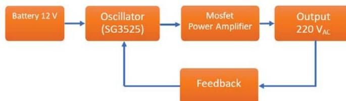
FIGURE 3. Composition of designed power inverter
