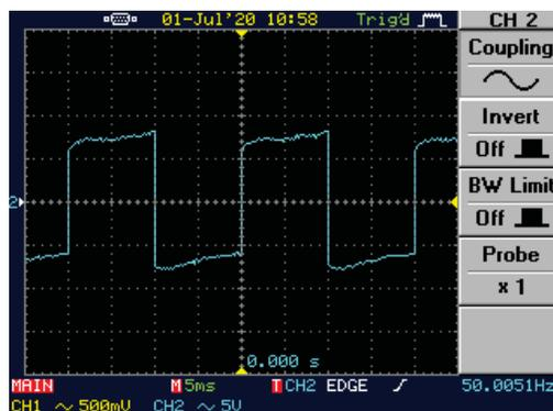
FIGURE 5. Result of output voltage of the IC SG3525 module
