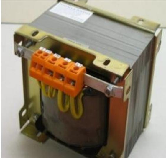
Gambar 8.7 Transformator tipe shell
