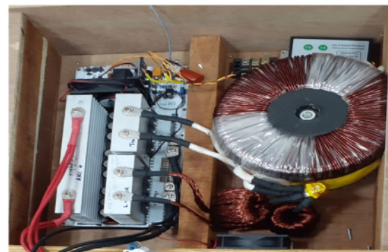
Fig. 9. Design of a SPWM Power inverter.
