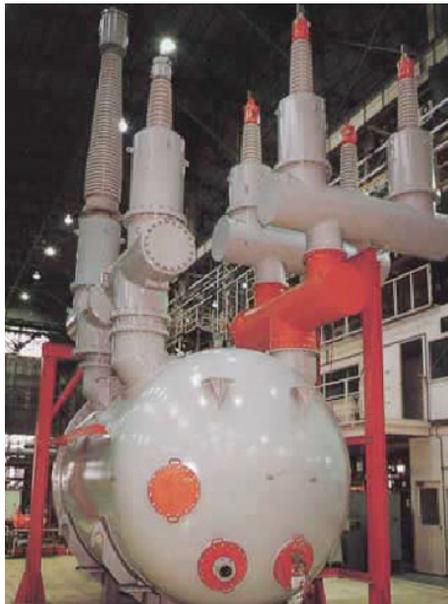
Gambar 8.1 Gas Insulated Switchgear.
