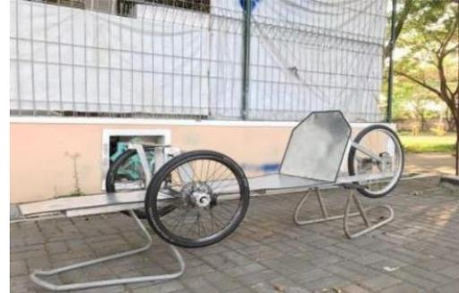
Gambar 2.2 Rangka *Prototype* Mobil Listrik
