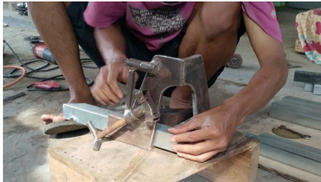
Gambar 4. 9. Proses Setup Menggunakan Three Axis Fixture Vise
