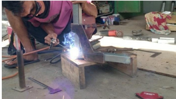
Gambar 4. 11. Proses Pengelasan Menggunakan Three Axis Fixture Vise
