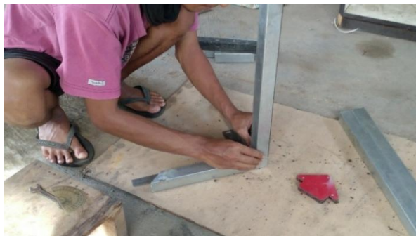
Gambar 4. 10. Proses Setup Tanpa Menggunakan Three Axis Fixture Vise
