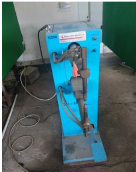
Gambar 2.2 Mesin spot welding
