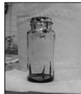
Fig. 1. A binder sample prepared for tank leaching test.
