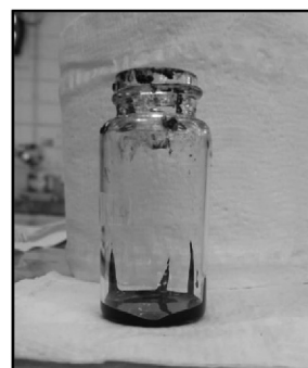
Fig. 1. A binder sample prepared for tank leaching test.
