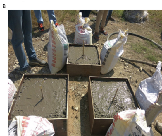
Fig. 2. (a) Concrete blocks with thermocouple; (b) Fixing the thermocouple.
