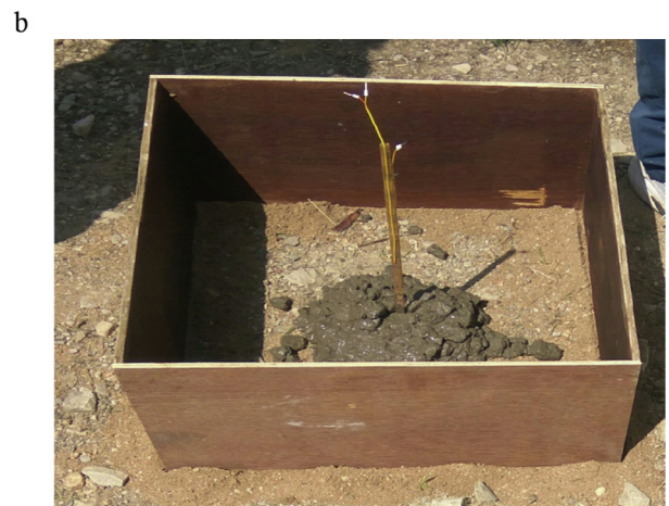
Fig. 2. (a) Concrete blocks with thermocouple; (b) Fixing the thermocouple.
