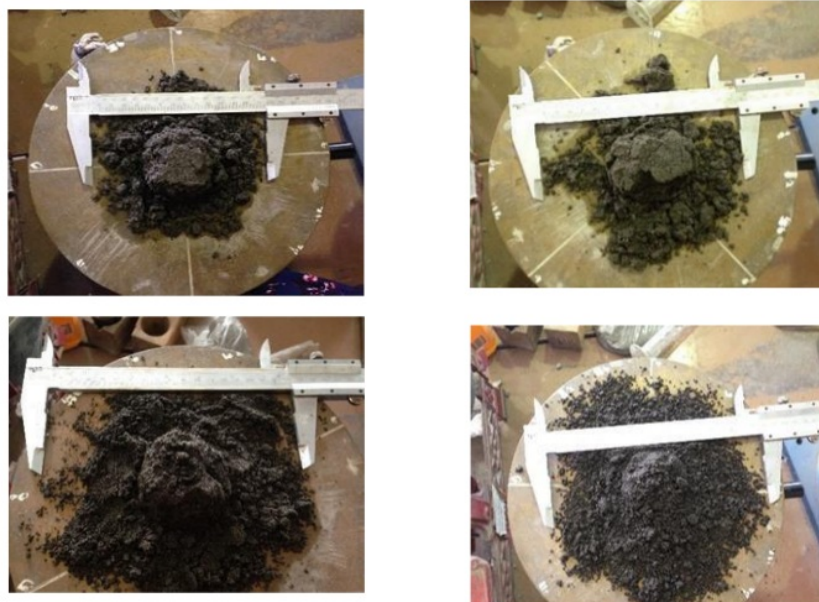
Figure 2. Flow test specimen (a) 100% Portland cement; (b) 25% palm oil ash; (c) 50% palm oil ash; (d) 75% palm oil ash
