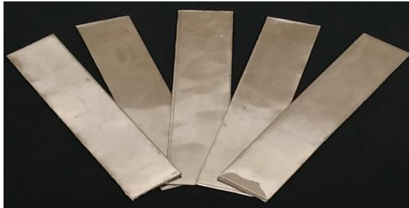
Gambar 3.2. Plat baja tahan karat Stainless steel 430
