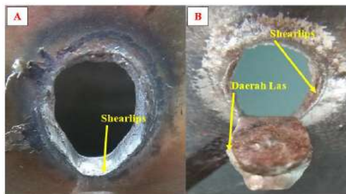
Gambar 2. 5 Foto makro pengelasan 1200 A (a)Stainless steel AISI 304 (b)Baja karbon rendah St 41. (Fachruddin, dkk. 2016)
