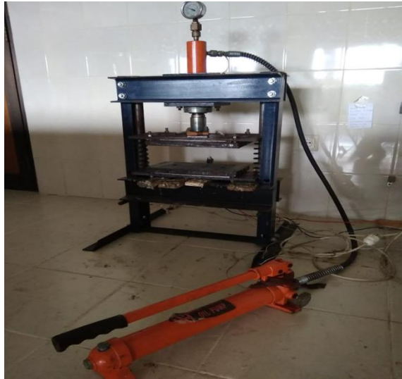
Gambar 3.8 Mesin cold press Molding
