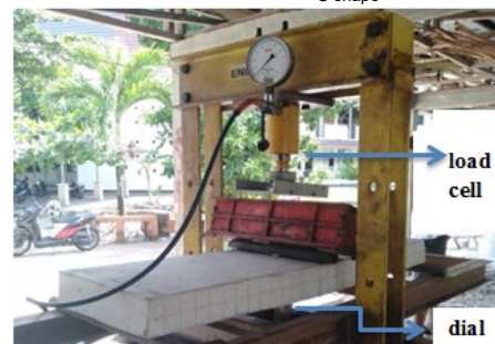
Fig. 4. Detail of slab and Set-up of test
