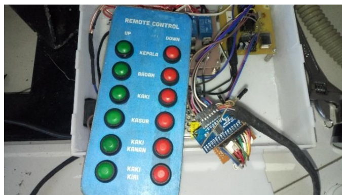
Gambar 3.9 Remote Control Push Button dan Multiplexer
