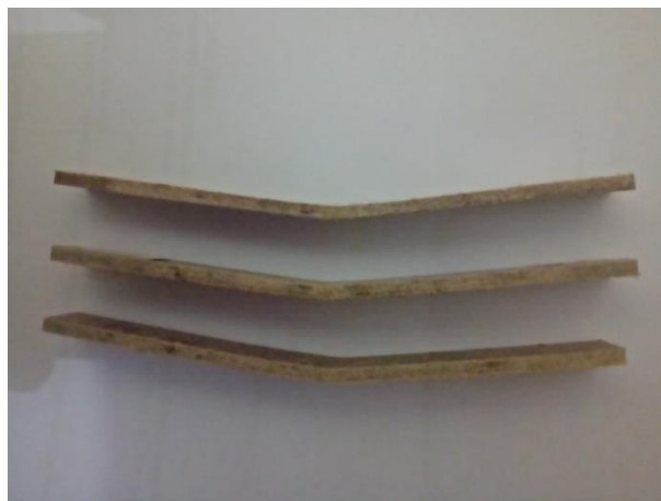
Gambar 4.4 Spesimen Hasil pengujian Bending ASTM D790
