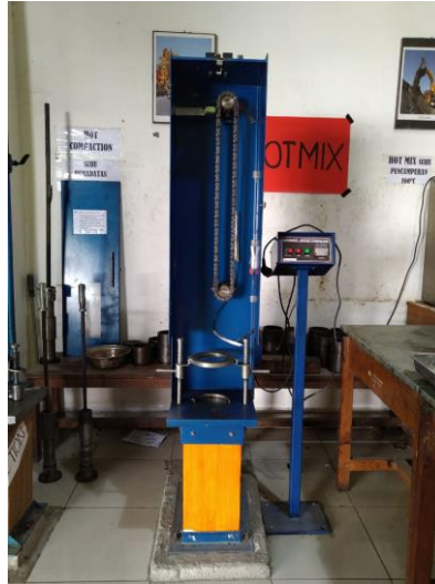
Gambar 3.11. Automatic Asphalt Compactor
