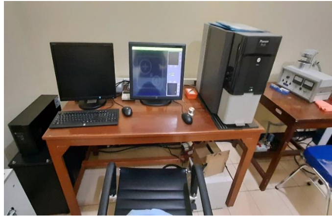
Gambar 3.7 Phenom ProX Desktop SEM
