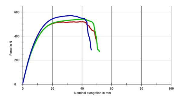
Customer : Sarwan Noor MPa Pre-load 0,1 Test standard : ASTM D 638 Speed, tensile modulus 50 mm/min 50 Material Nylon Test speed mm/min Notes : 3D Printing Tipe 5 Machine data : Zwick Z020 Grip to grip separation at the start position : Gage length, standard travel 115,00 mm
