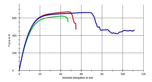
: Sarwan Noor Customer Pre-load 0,1 MPa Test standard: ASTM D 638 Speed, tensile modulus 50 mm/min : Nylon Test speed 50 mm/min Material Grip to grip separation at the start position: 115,00 mm
