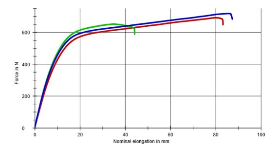
Sarwan Noor ASTM D 638 Customer Customer : Test standard : Pre-load 0,1 MPa Speed, tensile modulus 50 mm/min Material Nylon Test speed 50 mm/min Grip to grip separation at the start position :
