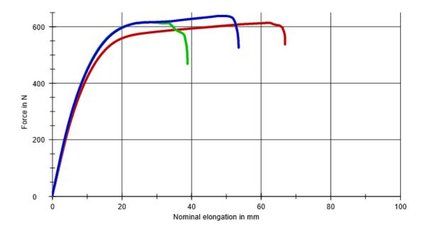
Customer : Sarwan Noor Pre-load 0,1 MPa Test standard: ASTM D 638 Speed, tensile modulus 50 mm/min Test speed 50 Material : Nylon mm/min Notes : 3D Printing Tipe 4
