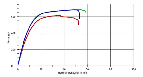
Customer : Test standard : : Sapwan Noor : ASTM D 638 MPa Pre-load 0,1 Speed, tensile modulus mm/min 50 Material Nylon Test speed 50 mm/min Grip to grip separation at the start position :
