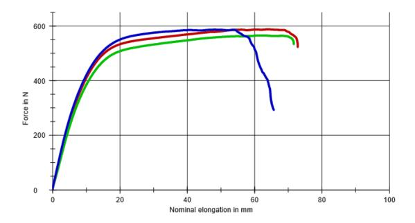
Customer Sarwan Noor Pre-load 0,1 MPa Speed, tensile modulus mm/min Test standard: ASTM D 638 50 Test speed 50 Material Nylon mm/min Notes : 3D Printing Tipe 3 Machine data : Zwick Z020 Grip to grip separation at the start position :
