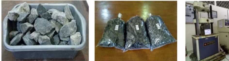
Figure 1. Ballast Aggregate, Scrap Rubber and Compressive Strength Testing Process with Universal Testing Machine
