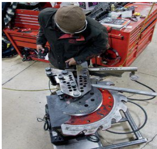
Gambar 3.10 Alat bending pipa
