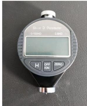
**Gambar 3.5** Alat Uji Kekerasan *Shore D Durometer*
