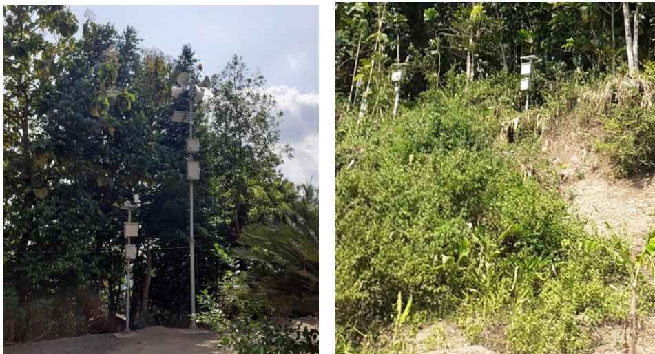
Gambar 15. Early Warning System (EWS) Longsor di Dusun Tambalan
