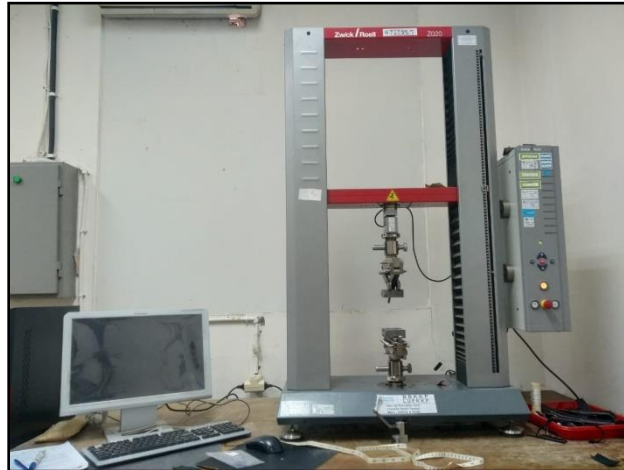
Gambar 3.5 Alat Uji Tarik Zwick Roell Z020
