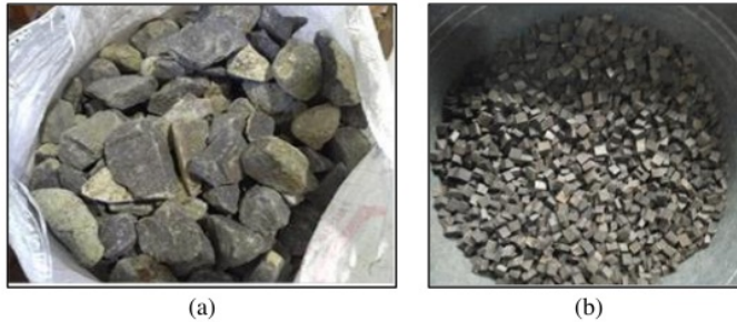
Fig. 1 - (a) Ballast materials; (b) Scrap rubber.
