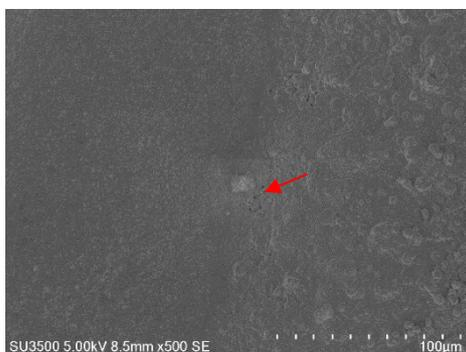
Gambar 2. Porositas sampel C2
