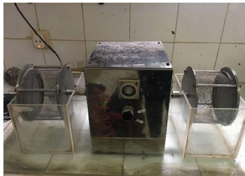
Gambar 3.5 Alat Uji *Slake durability*
