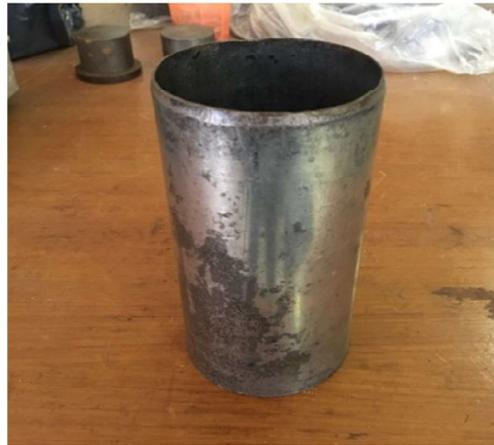
Gambar 3.2 *Mould* Uji Tekan Bebas
