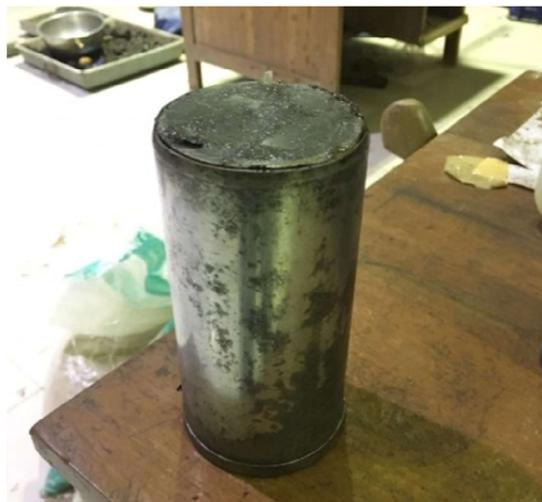
Gambar 3.3 *Mould* Uji Triaksial
