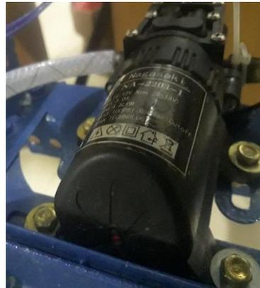
**Gambar 9** Pompa DC 12 V
