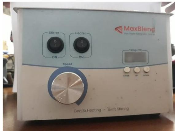
**Gambar 4.7** Hot plate magnetic steel
