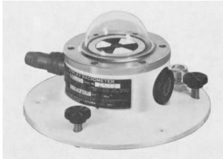
Gambar 2.9 *Pyranometer eppley black-and-white* (Duffie dkk, 2013)
