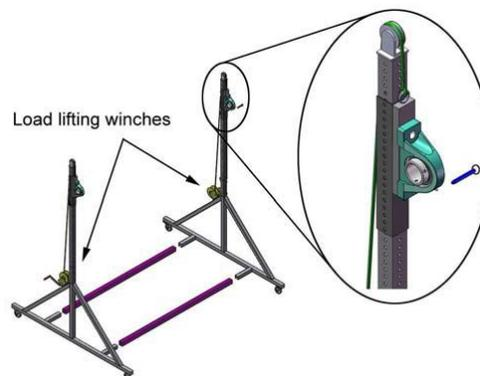
Gambar 2.7 *Load lifting winches* (Codd dkk, 2010)
