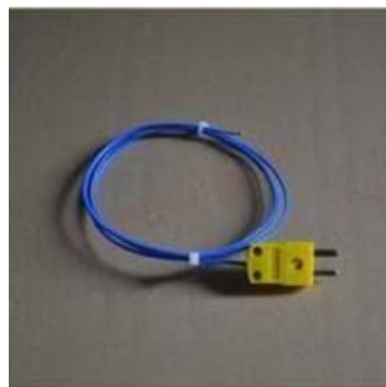
Gambar 3. 16 Termokopel tipe K
