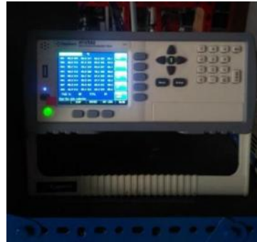
Gambar 3. 15 Applent Temperature Data Logger AT 4532
