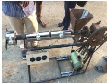
Gambar 2.1. Mesin Extruder rancangan harimalairajan (Harimalairajan dkk, 2016)
