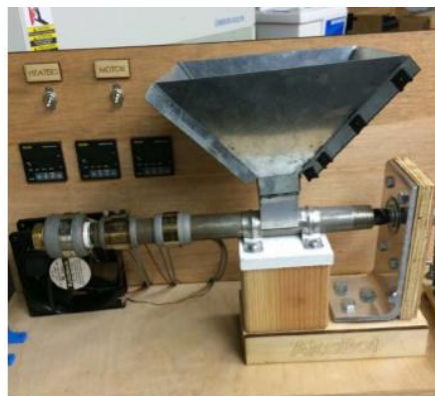
Gambar 2.4. Mesin Extruder rancangan Dubashi (Dubashi dkk, 2015)
