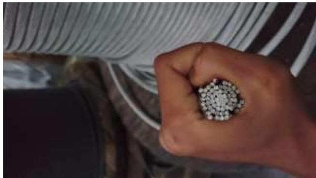
Gambar 2.2. Kabel A3C
