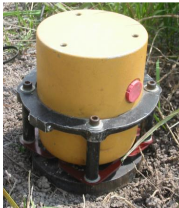
Gambar 4.6: Sumber harmonik-aktif electromagnet Ling Dynamics model 400
