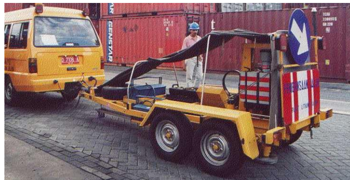
Gambar 5.22: Alat pengujian falling weight deflectometer
