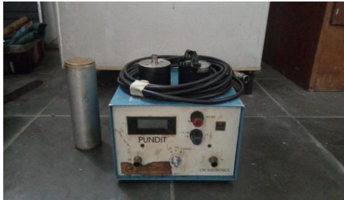
Gambar 3.21 UPVT ( Ultrasonic Pulse Velocity Meter)
