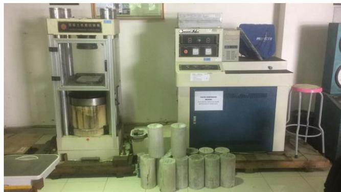
Gambar 3.19 *Concrete compression tester machine*
