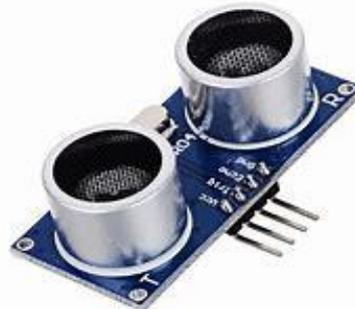
**Gambar 3.10** Sensor Ultrasonik
