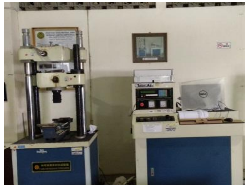
Gambar 3. 5 Flexural machine test
