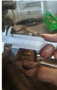
Gambar 4.11 Ukur ketebalan cakram
