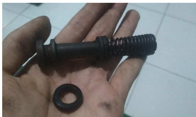
Gambar 4.24 Seal piston master rem
