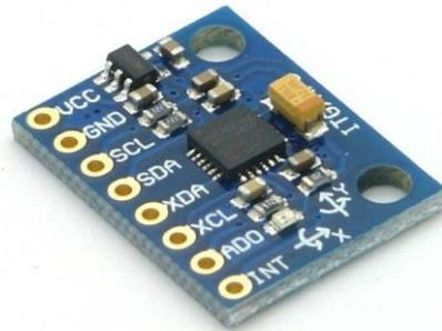
Gambar 2.1 Sensor *Accelerometer* MPU 60-50
