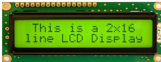
**Gambar 2.6** LCD 2x16 [8].
