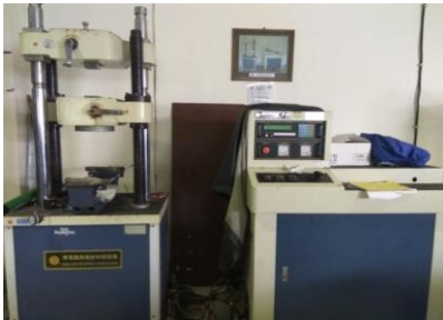
Gambar 1 Universal machine test Pengujian kuat tekan beton SCC
