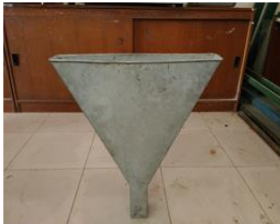
Gambar 15 Alat pengujian V-Funnel
