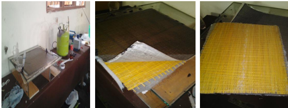
Gambar 3.6 proses vacum serat bambu
